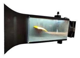
Our fully 3D-printed Desktop Wind Tunnel offers precise airflow visualization around objects. It comes with airfoil, cylinder, and flat plate attachments, using dhoop as a smoke generator for clear flow patterns—ideal for hands-on aerodynamics learning and experiments.
